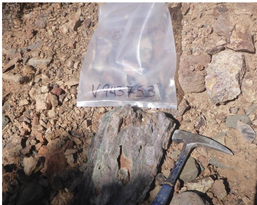
Figure 41: Sample of gray quartz veining and silicification from adit dump (V943753)
