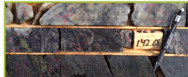
Core Sample at Reef Gold hosted in quartz-sulfide veins and stringers cutting sheared mafic volcanic and gabbroic rocks
