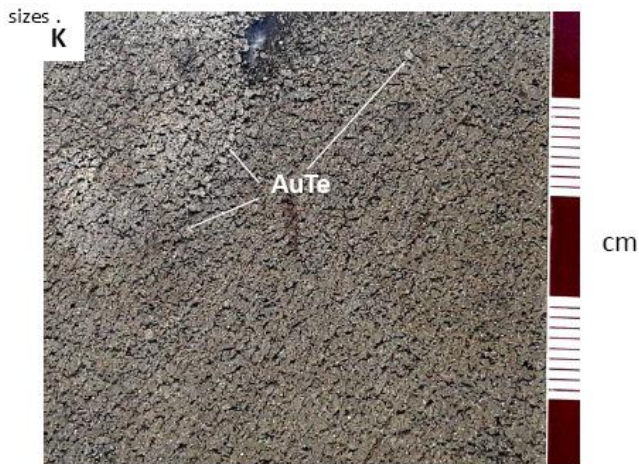
Polished core from DDH-B90-4, ~580m. Fine-grained, massive, intergranular-textured massive sulfide (auriferous pyrite) in the lower massive sulfide lens. Note very fine-grained interstitial (white-color) gold tellurides (AuTe) grains scattered in pyrite matrix. This sample assayed 3.1g/t Au, 1.1g/t Ag and 0.07% Cu over ~1 meter.
