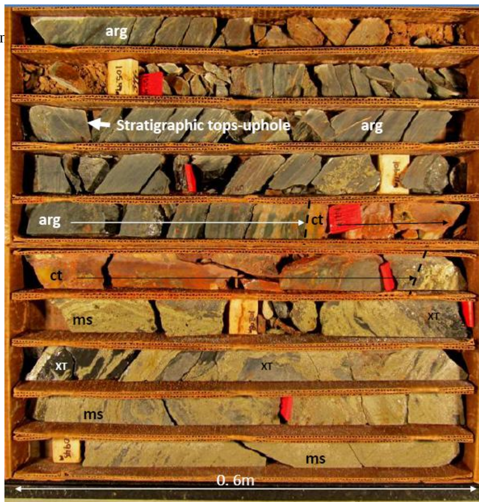
Photograph G Drillhole intercept (DDH-B12-01) of the upper massive sulfide lens (ms) . This interval from 107.7 - 110.4 meters assayed 2.85% Cu and 0.42g/t Au over 2.7
